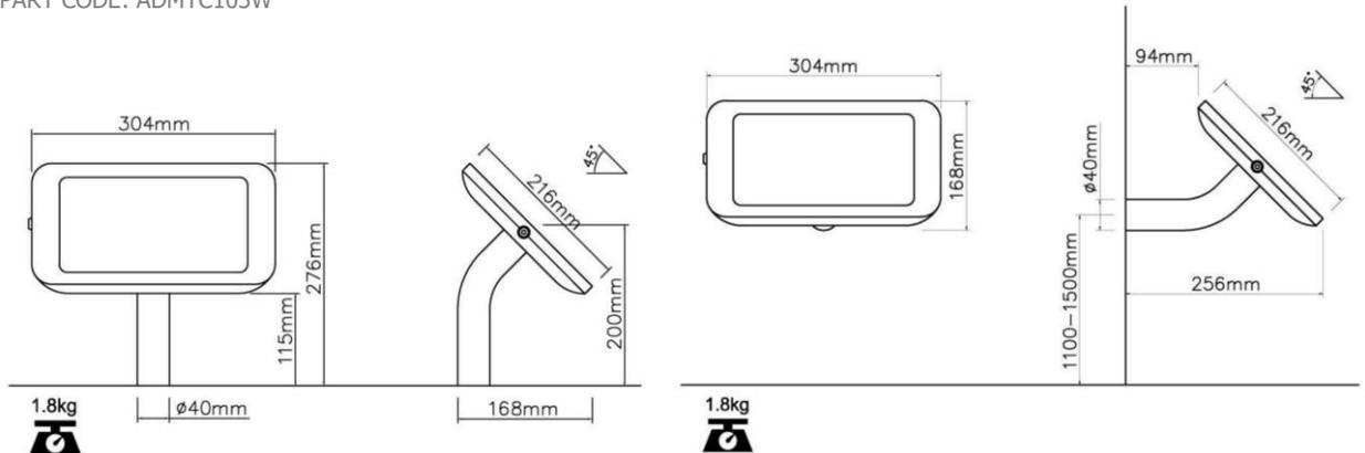
**LocPad® 60° mounting tube.** The 60° angled tube can be mounted onto a desk or wall.
