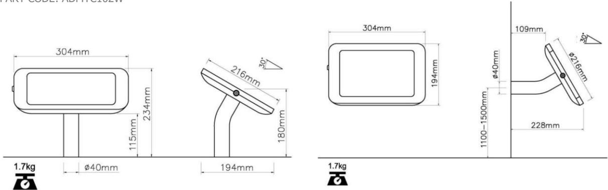
**LocPad® 45° mounting tube.** The 45° angled tube can be mounted onto a desk or wall and has is the best 'all round' choice for most installations. If you're not sure which mount to use, the 45° mounting tube is usually the one to go for.
